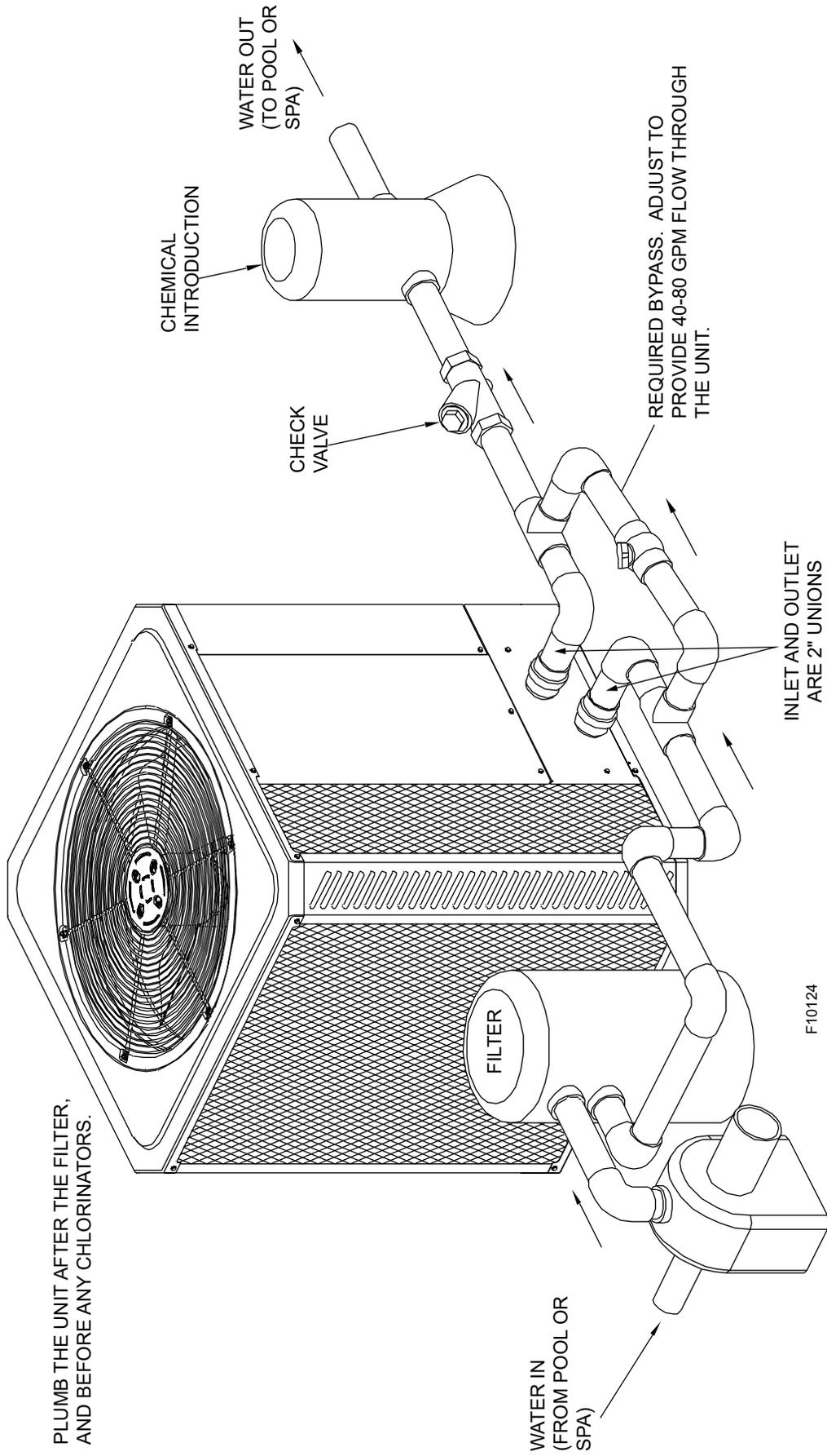
Figure 9. For Systems with Flow over 80 GPM (303 lpm)
