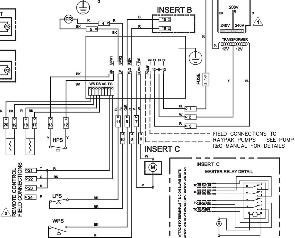
3. FOR 2 WIRE REMOTE CONTROL: USE TERMINALS 21 & 22 TO ATTACH 2 WIRE CONTROL SYSTEMS THAT HAVE THEIR OWN SENSORS FOR TEMPERATURE CONTROL. SET POOL TEMPERATURE TO OFF AND SPA TEMPERATURE TO 104°.
