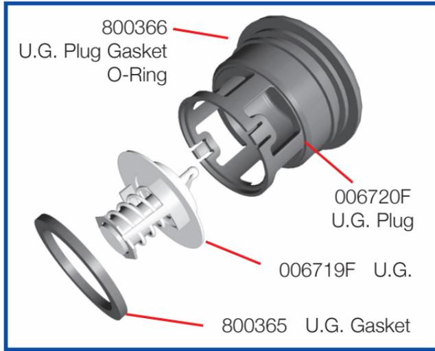
**Tech Tip:** Test a U.G. by placing it in a bowl of hot water. If working properly, it will open as it warms up.
