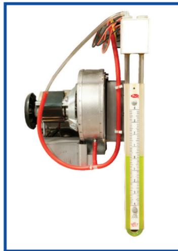
**How to read pressure on Low NO<sub>x</sub> Fan.**
