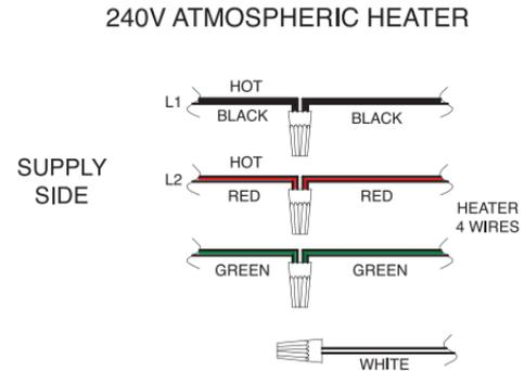
Note: Heater will not work properly if wired to a 208VAC power source.
