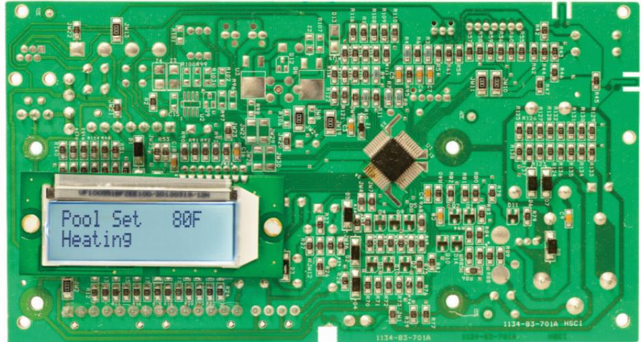
Advanced Flame Technology (AFT) printed circuit board.
