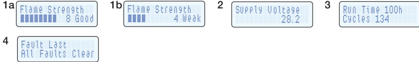
Service Displays provide critical performance data on the operation of the heater. This information can be viewed from Off, Pool, Spa and Remote Modes by pressing the UP button and the mode button for 3 seconds.
