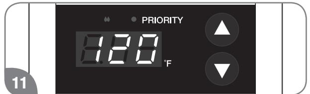
**11** Press the UP or DOWN adjustment button to set the desired temperature.
