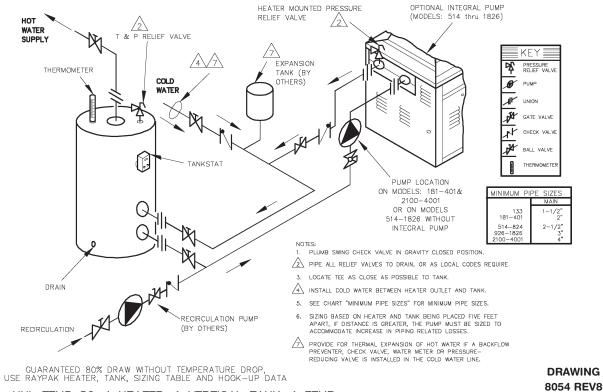
PIPING: UNI-TEMP 80, 1 HEATER, 1 VERTICAL TANK, 1 TEMP
