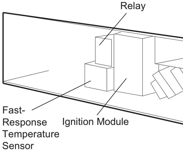
**Fig. 25: Control Box Component Locations Models 0135 & 0180**
