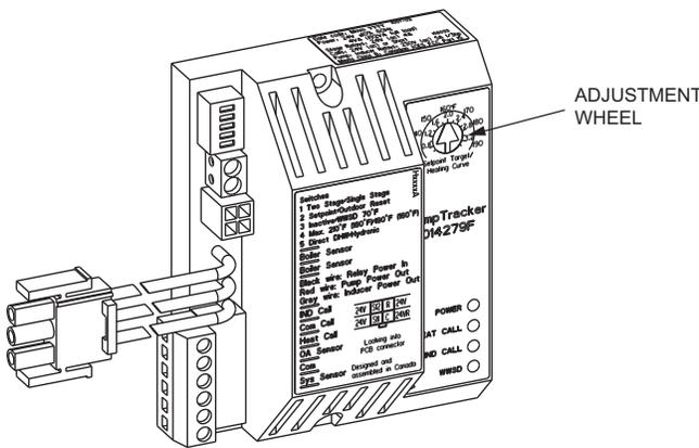
Fig. 15: Temperature Controller
