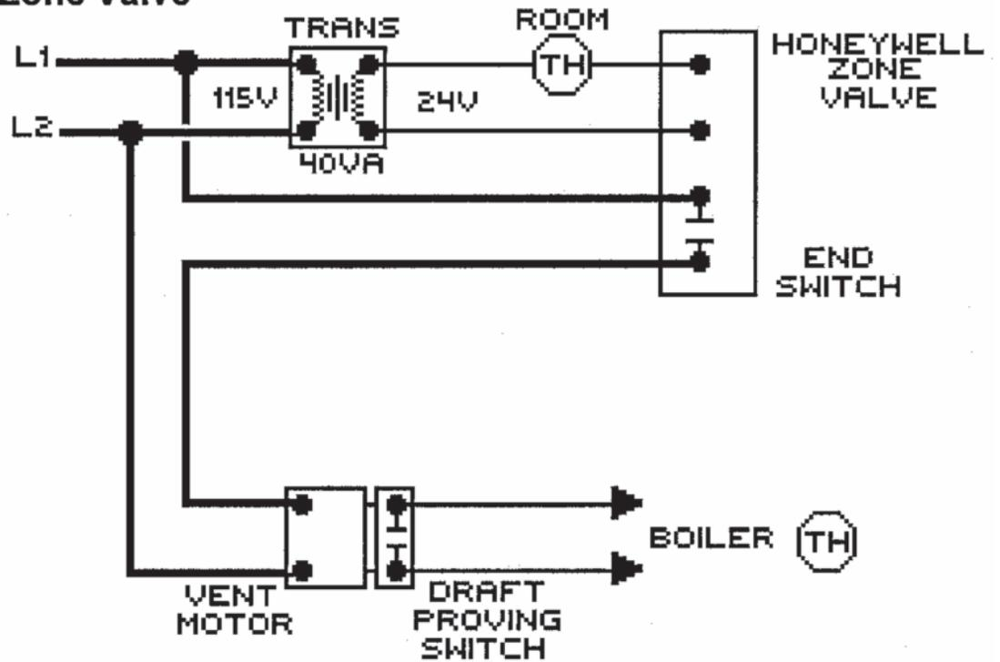
Fig. 24: Power Vent System with Zone Valve (Honeywell)
