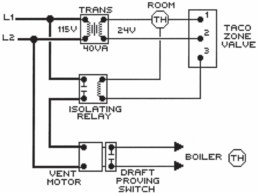
Fig. 23: Power Vent System with Zone Valve (Taco)
