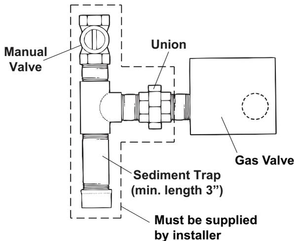
Fig. 14: Sediment Trap
