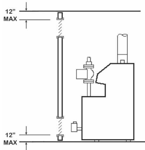
**Fig. 3: Location of Openings for Combustion/Ventilation Air**
