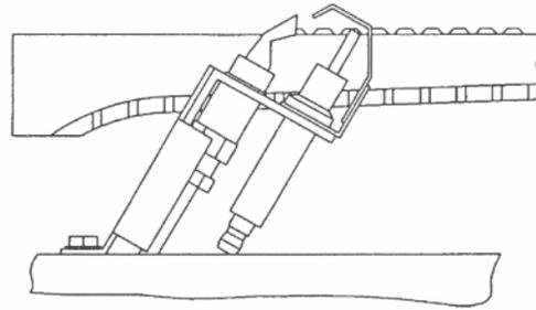
**Fig. 29: Honeywell Pilot**
