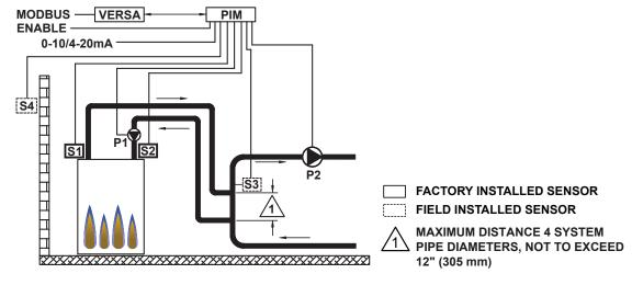
Figure 10. Mode 1 - Single Heater with Primary Secondary Piping
