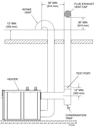
Figure 29. Direct Vent - Vertical
