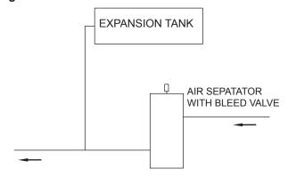
Figure 7. Air-Separation/Expansion Tank
