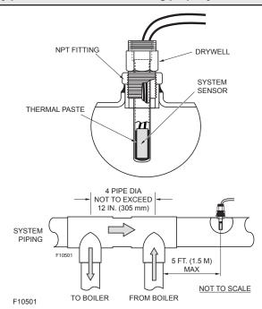
Figure 8. System Sensor Installation
