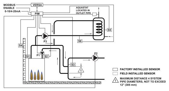
Figure 12. MODE 3 - Single Boiler with Indirect on Boiler Loop
