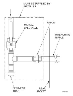
Figure 14. Gas Supply Connection
