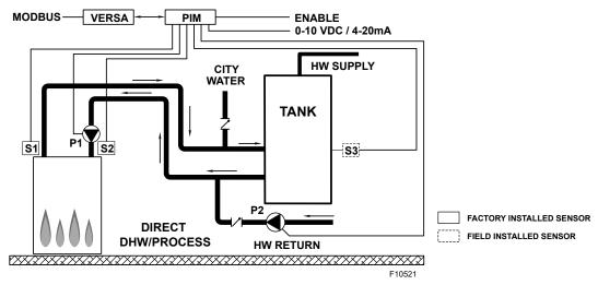
Figure 13. WH Units - Single Water Heater with Tank H Units - Single Boiler with Process Tank
