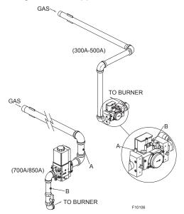
Figure 44. Gas Pressure Measurement Locations
