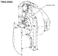
Figure 45. Pressure Vent Switch Assemblies
