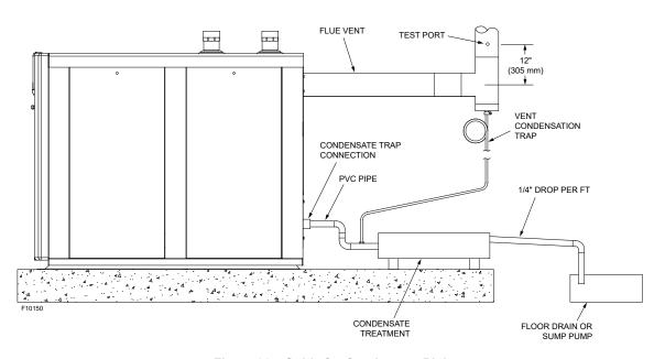
Figure 30. Guide for Condensate Piping
