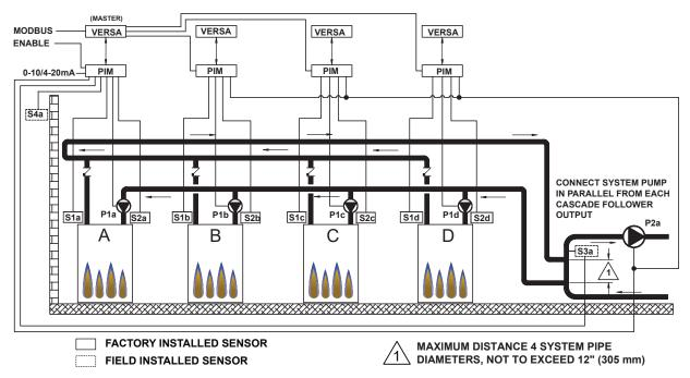
Figure 9. MODE 1 - Hydronic Multi-Boiler
