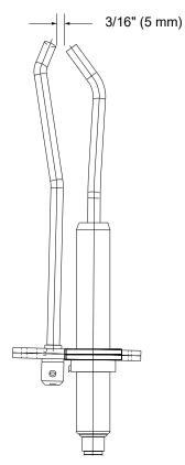
NOTE: If receiving a NO FLAME, check the gap spacing between the points on the electrode by using either a 3/16 drill bit or a key between the gap. There should be no resistance.
