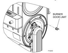
Figure 41. Burner Door Limit
