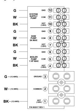
Figure 22. XFyre Cascade Master Pumps
