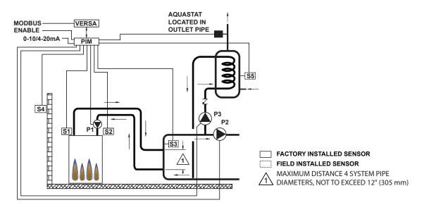
Figure 11. MODE 2 - Single Boiler with Indirect on System Loop
