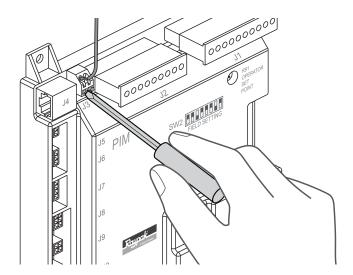
Figure 21. FT\_BUS Wire Connection
