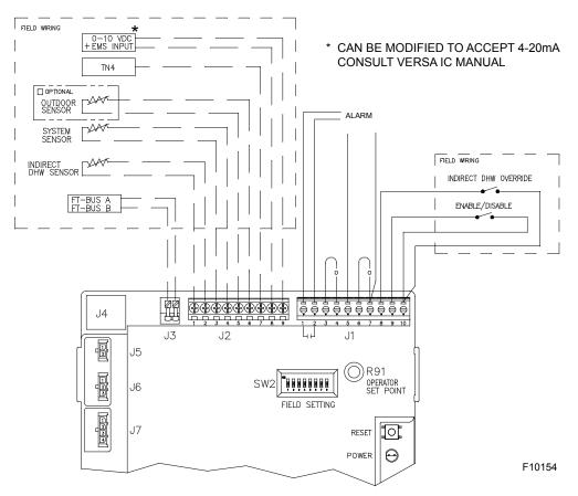
Figure 17. XFyre Single Heater Control
