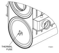
Figure 40. Thermal Fuse
