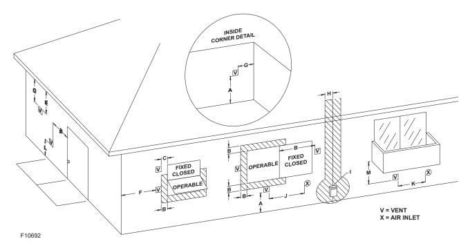
Figure 6. Minimum Clearances from Vent/Air Inlet Terminations – Indoor and Outdoor Installations
