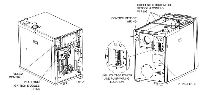
Figure 15. Front Wiring Locations
