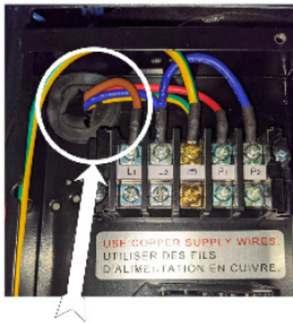
Figure 20. Insert Cable to PC Board (On/Off Models Only)
