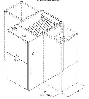
THE RXGR-C24B MUST ONLY BE INSTALLED ON THE SIDE OPPOSITE THE GAS AND ELECTRICAL CONNECTIONS.
