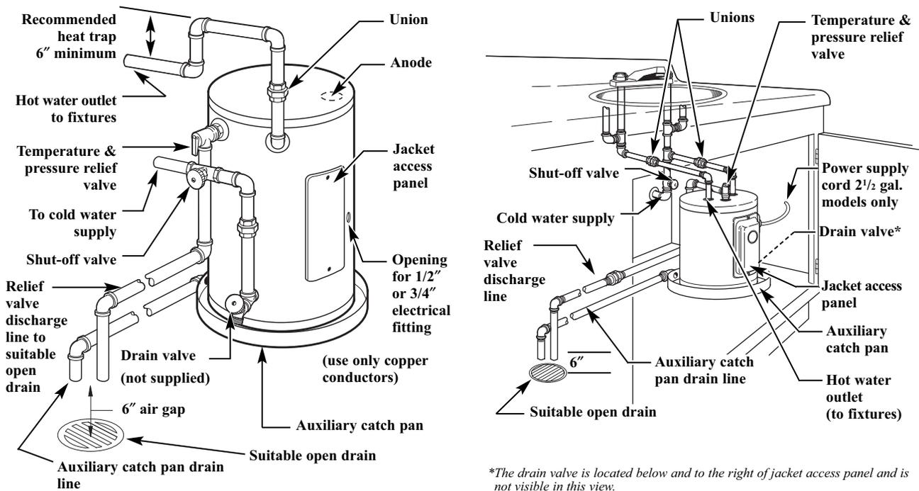
A new combination temperature and pressure relief valve, complying with the Standard for Relief Valves and Automatic Gas Shut-Off Devices for Hot Water Supply Systems, ANSI Z21.22, is supplied and must be installed in the opening provided and marked for the purpose on the water heater. No valve of any type should be installed between the relief valve and the tank. Local codes shall govern the installation of relief valves.
