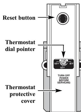
The illustration at the left shows the temperature adjustment dial used for setting the water temperature.
