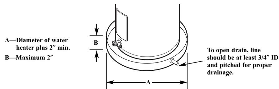
**NOTICE: Auxiliary catch pan MUST conform to local codes.**
