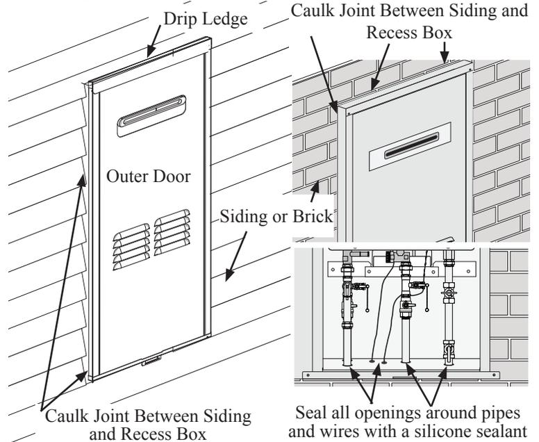
**Warning** - All openings in the bottom of the recess box must be sealed to prevent water infiltration in to the wall. Failure to do so could result in damage to the wall.
