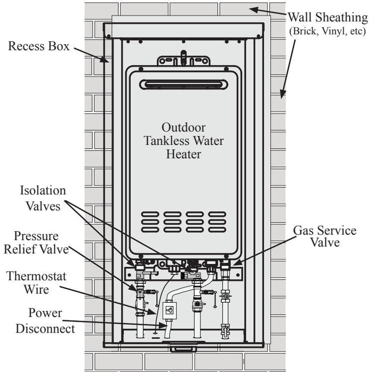
**Final Assembly and Inspection** - Follow the Use and Care Manual for complete details about the water heater. Check all water and gas connections for leaks.
