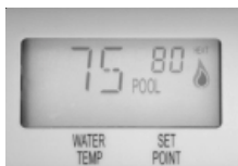
Heating in the POOL Mode
