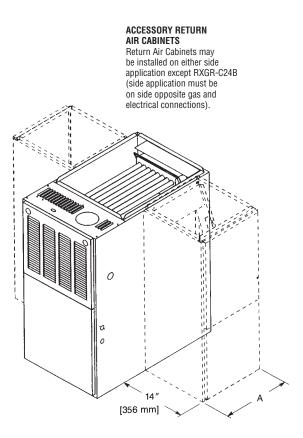
THE RXGR-C24B MUST ONLY BE INSTALLED ON THE SIDE OPPOSITE THE GAS AND ELECTRICAL CONNECTIONS.
