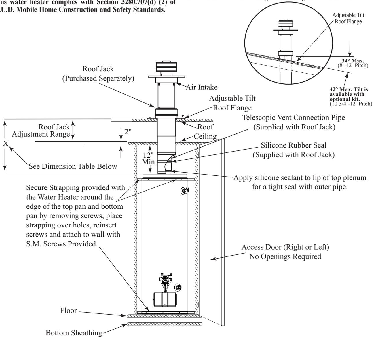
Secure Strapping provided with the Water Heater around the edge of the top pan and bottom pan by removing screws, place strapping over holes, reinsert screws and attach to wall with S.M. Screws Provided.
