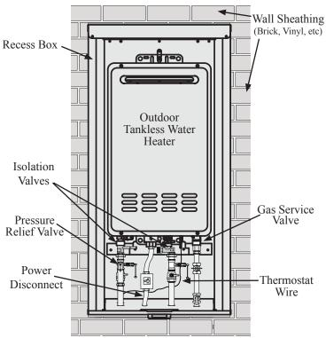
**Final Assembly and Inspection** - Follow the Use and Care Manual for complete details about the water heater. Check all water and gas connections for leaks.
