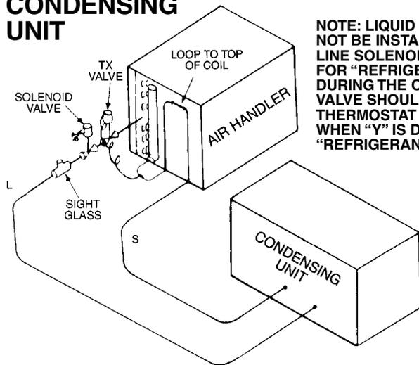
**NOTE: LIQUID LINE SOLENOID VALVE MUST NOT BE INSTALLED FOR PUMP DOWN. LIQUID LINE SOLENOID VALVE MAY BE INSTALLED FOR "REFRIGERANT ISOLATION" ONLY DURING THE OFF-CYCLE. THE SOLENOID VALVE SHOULD BE CLOSED WHEN THE THERMOSTAT IS SATISFIED (VALVE CLOSED WHEN "Y" IS DE-ENERGIZED) FOR EFFECTIVE "REFRIGERANT ISOLATION".**
