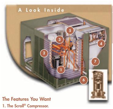
All of our residential package units - regardless of efficiency level – feature the Scroll Compressor. The scroll compressor uses a more advanced technology than traditional reciprocating compressors. They have fewer moving parts, and they are quieter, more efficient, and longer lasting.
