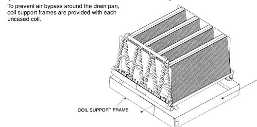
Frame is only used when coil is not installed in other than standard coil casing. Air bypass frame is not for use with TXBC coil casing or AH series air handlers.
