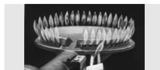
Proper burner and pilot burner pattern.
