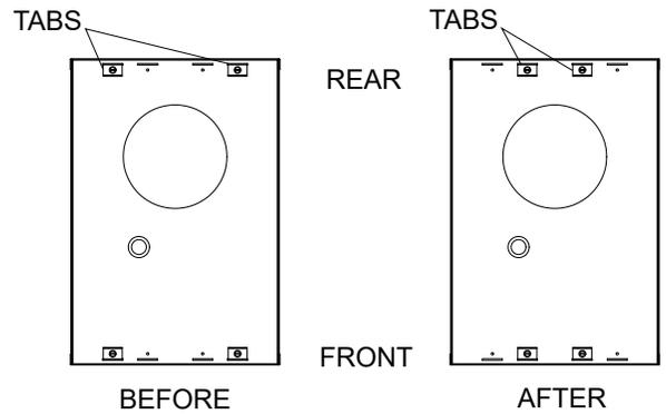
**Figure 1. Position of Mounting Tabs**
