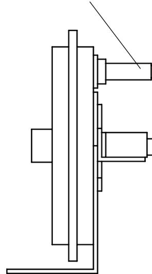
Figure 6. Draft Proving Switch
