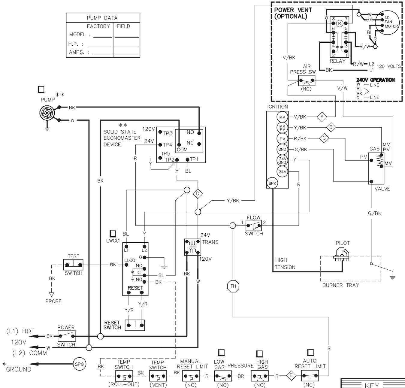
**NOTES: \*** USE GROUND CONNECTION PROVIDED. FAILURE TO PROVIDE PROPER GROUND MAY RESULT IN LOCK-OUT ALL GROUND  $\perp$  TERMINATE AT  $\text{SPG}$ .
