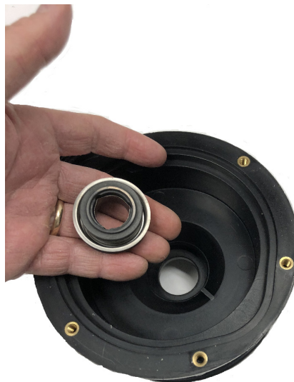
Figure 14. Pump Volute Seal
