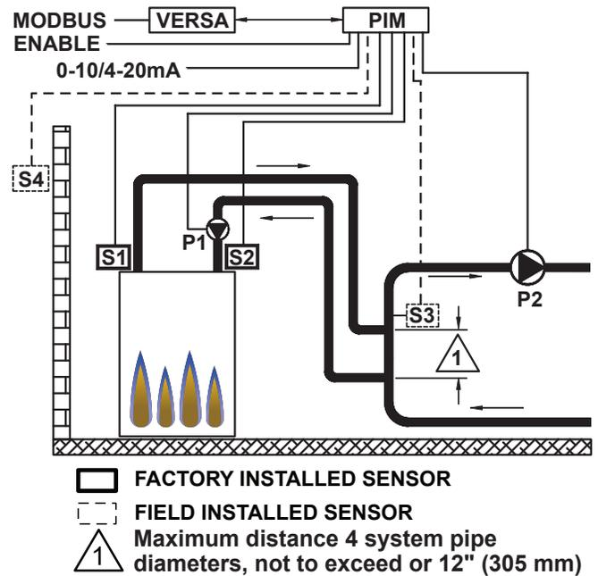
Figure 13. MODE 1 - Single Boiler with Primary/Secondary Piping
