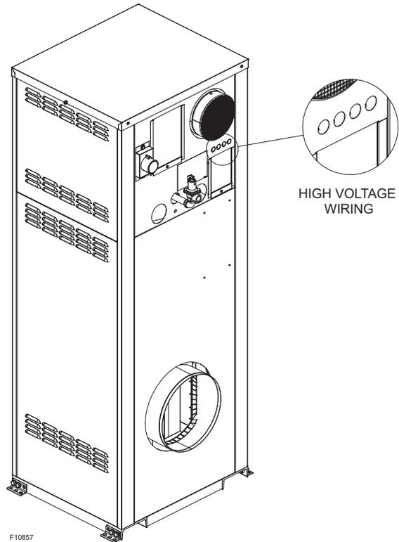
Figure 22. Wiring Location
