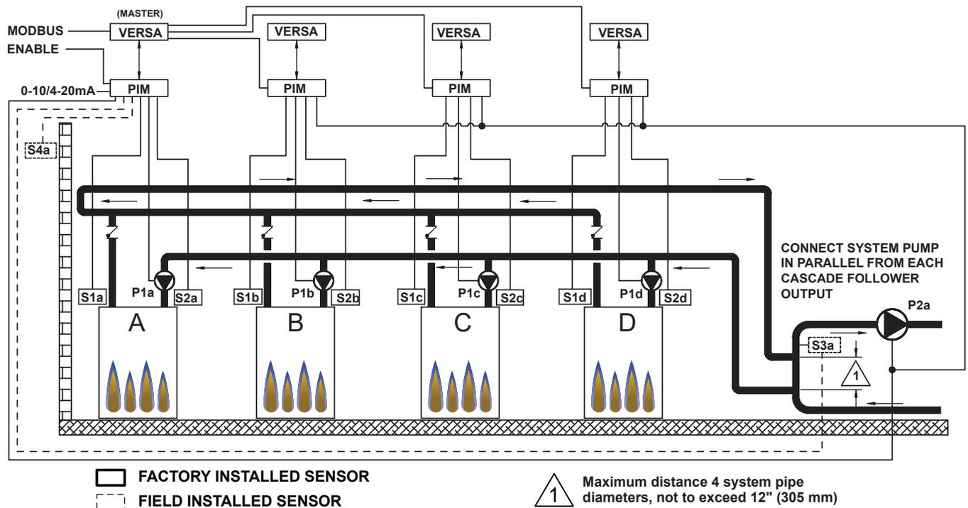
Figure 14. MODE 1 - Boiler Cascade with Primary/Secondary Piping
