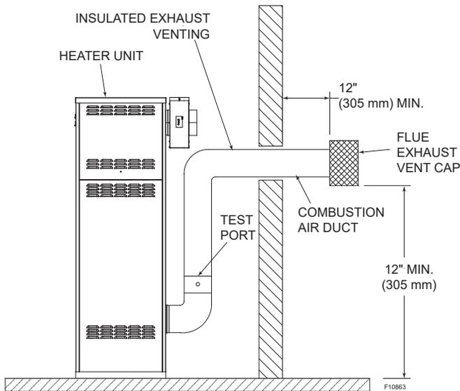
**Figure 30. Horizontal Through-the-Wall Venting with Ducted Combustion Air**
