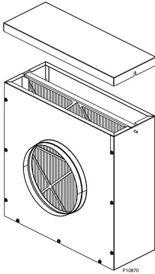
**Figure 47. Remove the Air Filter Box Cover**
