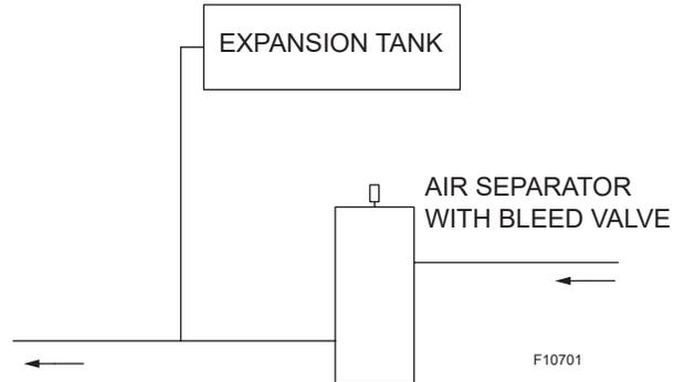
**Figure 12. Air-Separation/Expansion Tank**
