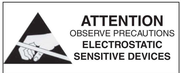
**NOTE:** Electrostatic Discharge (ESD) damage can be caused by direct or indirect contact with the wiring or circuit board. When one walks to the heater area, an electrostatic charge accumulates on the body. Contact of a finger allows the body to discharge, possibly causing device damage. This damage can be limited if the service person discharges himself, following ESD preventive/removal practices, and holds on to the heater enclosure for 5 seconds before proceeding.
