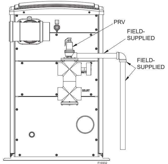
Figure 19. PRV Piping
