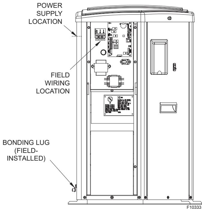
Figure 20. Wiring Locations
