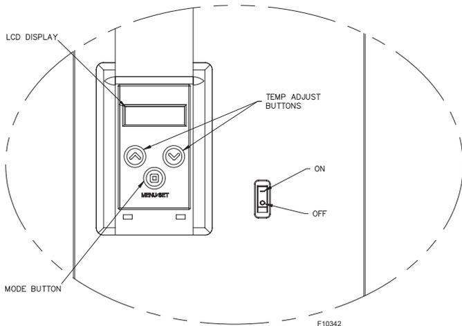
Figure 29. Control Adjustments
