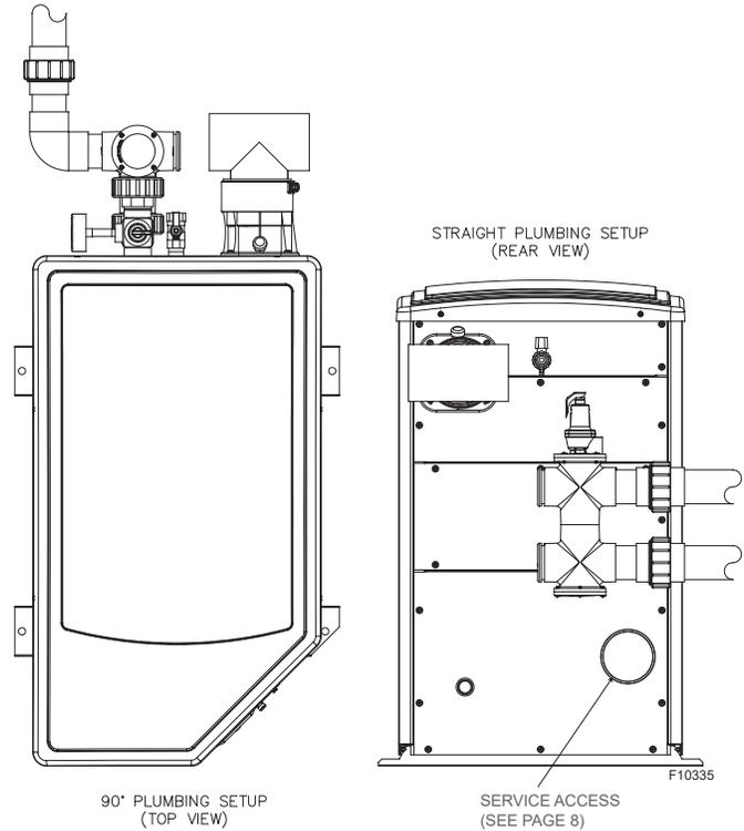
Figure 23. Plumbing Setup
