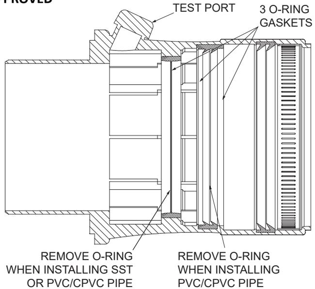
**Figure 13. Multi-Vent Adapter**
