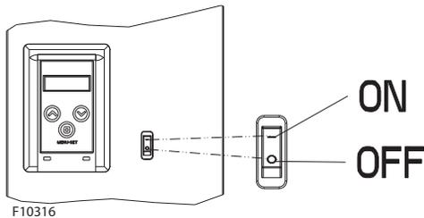
**Figure 44. Heater Toggle Switch**
