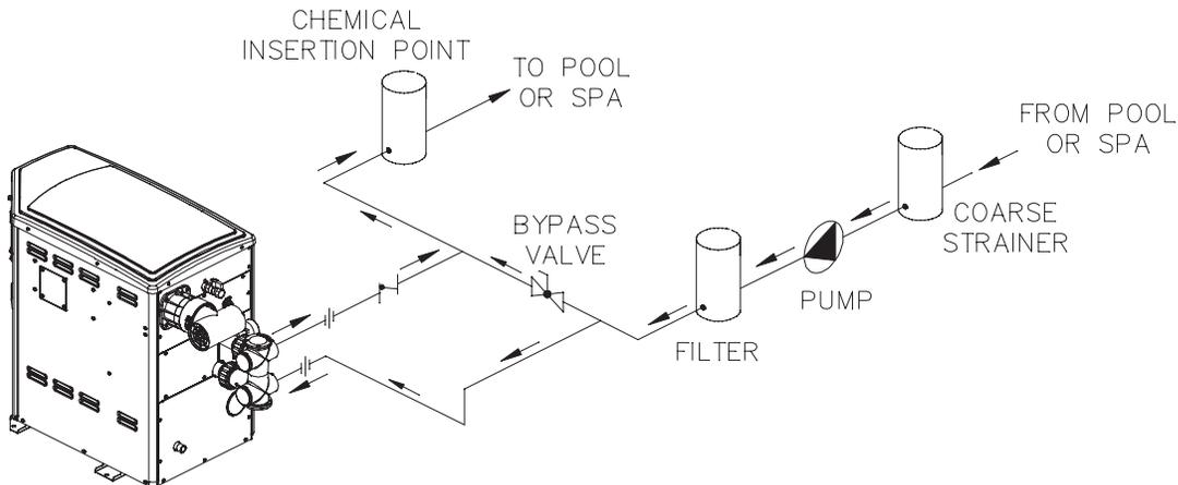
Figure 24. Single Pool or Spa Heater Installation
