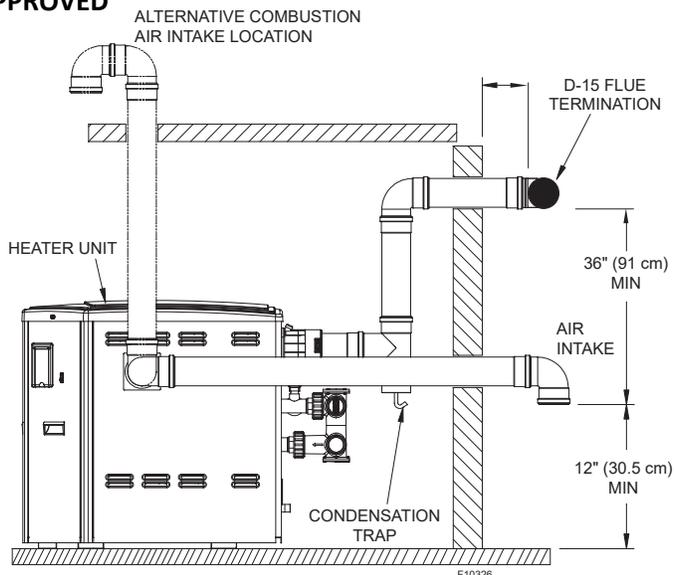
Figure 9. Horizontal Through-the-Wall Direct Venting
