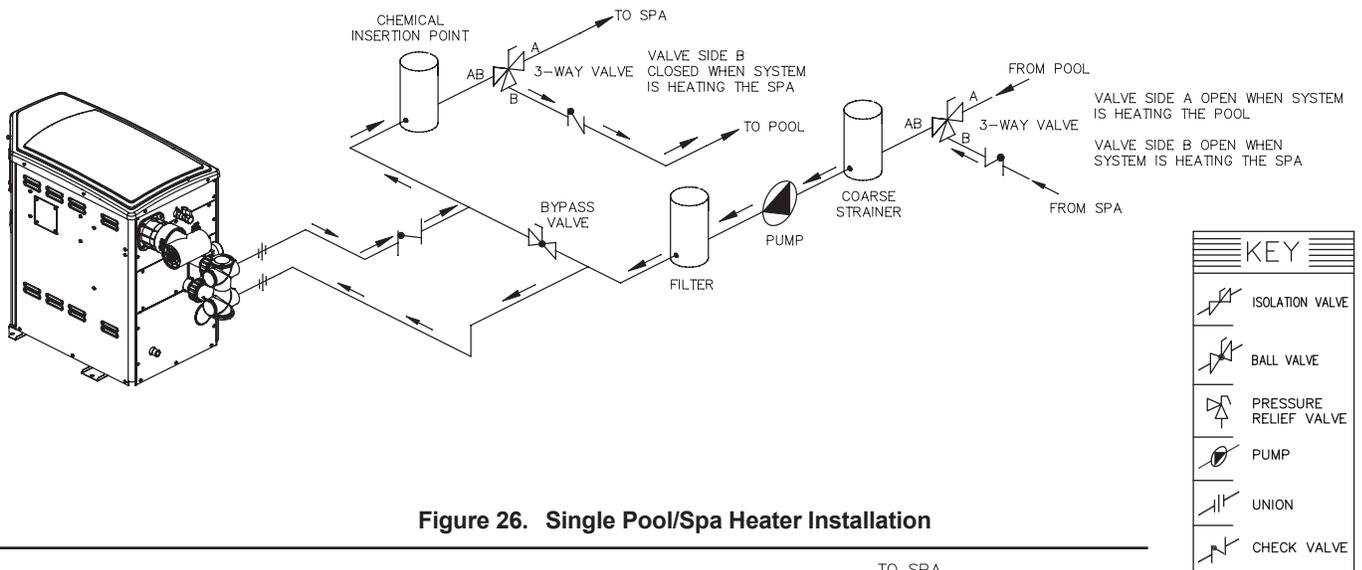
**Figure 26. Single Pool/Spa Heater Installation**
