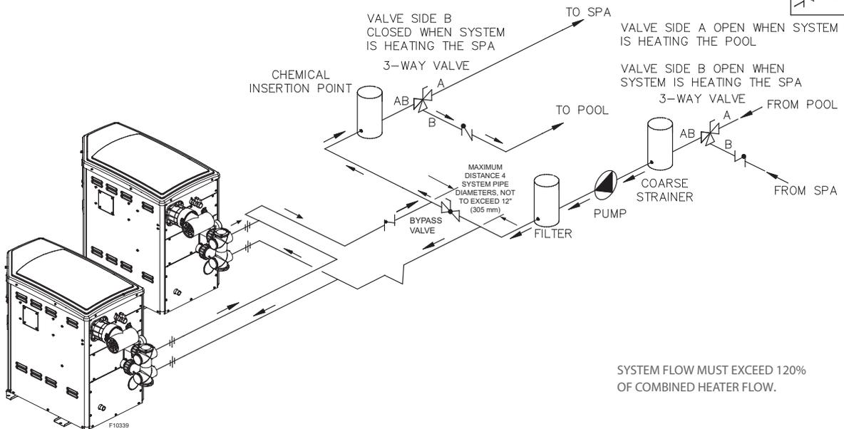
**Figure 27. Multiple Pool/Spa Heaters Installation**
