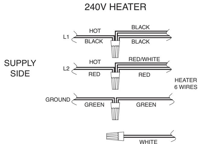
The heater must be electrically grounded and bonded in accordance with local codes, or, in the absence of local codes, with the latest edition of the National Electrical Code, ANSI/NFPA 70. (Canada - Canadian Electrical Code, CSA C22.1, Part 1 and Part 2.)
