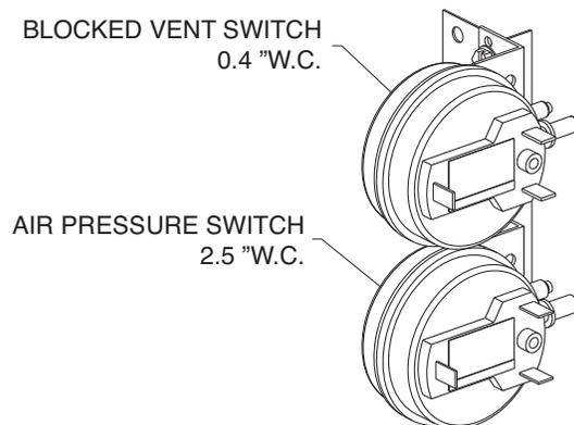
Air Pressure & Blocked Vent Switches
