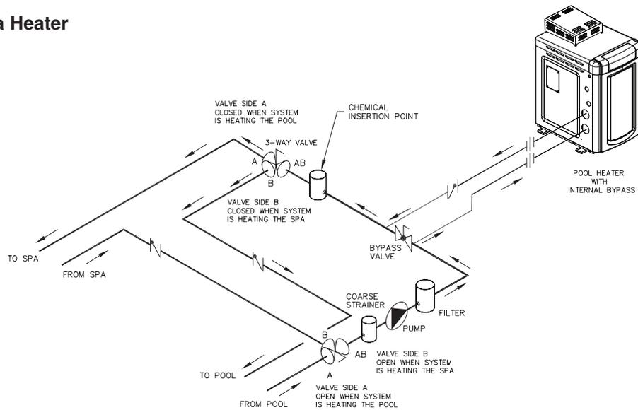
THIS DIAGRAM IS RAYPAK'S RECOMMENDATION AND IS NOT INTENDED TO REPLACE AN ENGINEERED PIPING SYSTEM BY A PROFESSIONAL ENGINEER.
