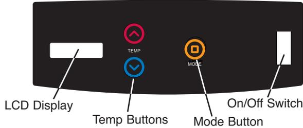
The pool heater touchpad, located on the upper front panel of the heater, allows the user to select either POOL or SPA operation, and to adjust the setpoint temperature. The LCD display window indicates the mode (OFF, SPA, POOL) and the actual water temperature. A manual power switch provided turns the control power ON or OFF.
