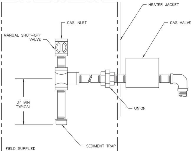
Gas piping must have a sediment trap ahead of the heater gas controls, and a manual shut-off valve located outside the heater jacket. All gas piping should be tested after installation in accordance with local codes.
