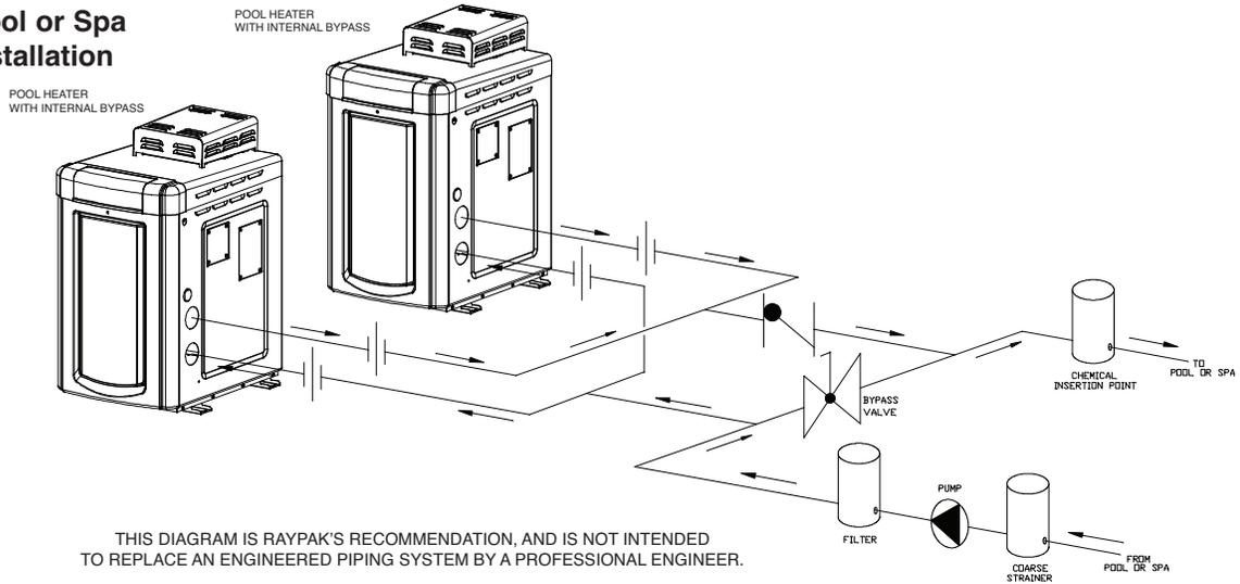
THIS DIAGRAM IS RAYPAK'S RECOMMENDATION, AND IS NOT INTENDED TO REPLACE AN ENGINEERED PIPING SYSTEM BY A PROFESSIONAL ENGINEER.
