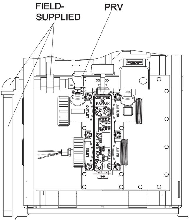
**NOTE:** To avoid water damage or scalding due to valve operation, drain pipe must be connected to valve outlet and run to a safe place of discharge. Drain pipe must be the same size as the valve discharge connection throughout its entire length and must pitch downward from the valve. No shut-off valve shall be installed between the relief valve and the drain line. Valve lever should be tripped at least once a year to ensure that waterways are clear.
