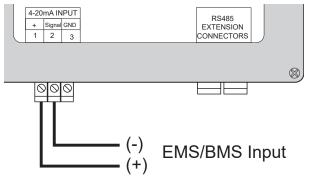
Figure 2. TempTracker Provides Current for 4-20 mA Signal
