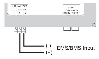
Figure 1. External Device (e.g. BMS) Provides Current for 4-20 mA Signal
