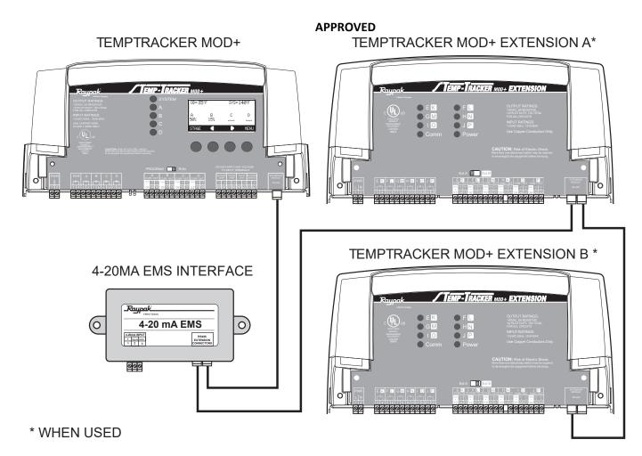
Figure 3. Connecting 4-20mA EMS Interface to TempTracker Mod+ with Two Extension Panels using RS485
