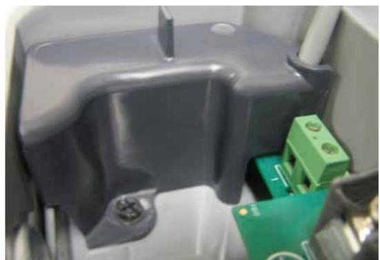
**Figure 21** - Plastic Cover Installed in Terminal Box
