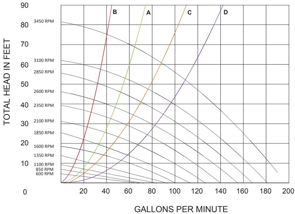
B, A, C, and D represent average system curves for pools with the pipe diameter mentioned below.
