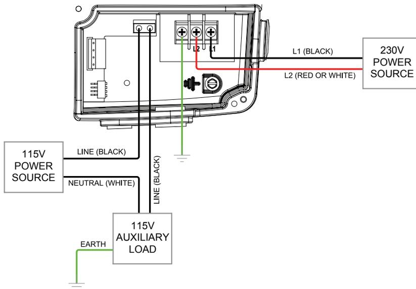
**Figure 4** - Wiring Diagram with 115V AUX Load
