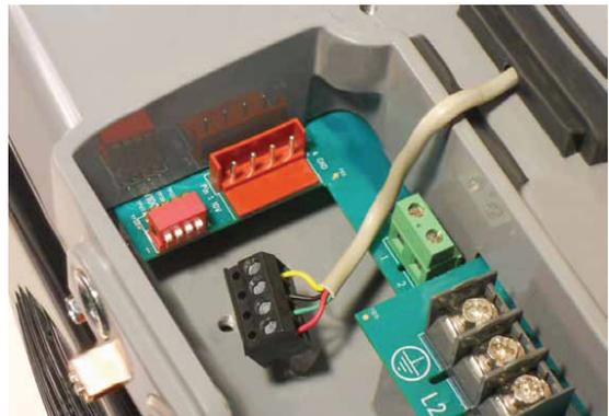
**Figure 19** - Communication Connector Removed
