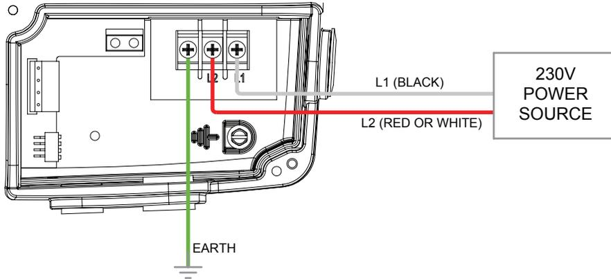
**Figure 3** - Wiring Diagram without AUX Load
