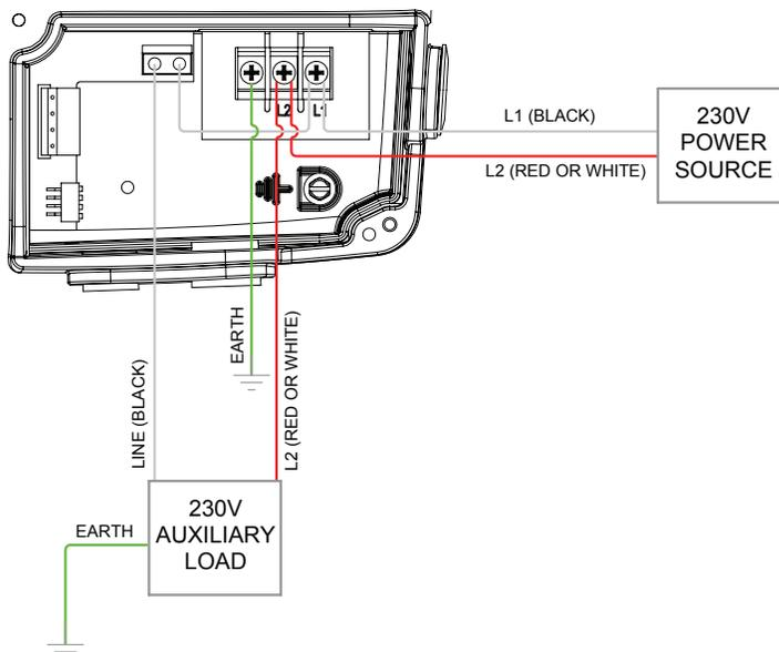
**Figure 5** - Wiring Diagram with 230V AUX Load
