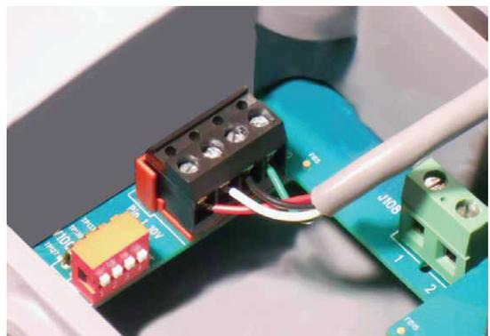
**Figure 20** - UI Connector Installed
