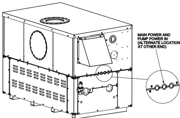
**Figure 31. Wiring Location**
