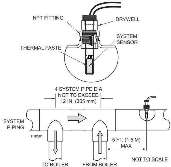
**Figure 15.** System Sensor Installation
