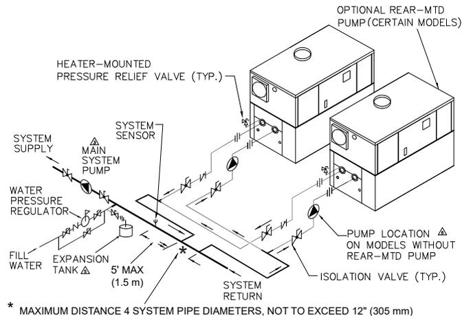
Figure 19. Dual Heaters (Reverse/Return) with Primary/Secondary Piping
