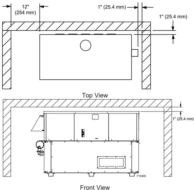
**Figure 6. Minimum Clearances from Combustible Surfaces – Indoor Installations**
