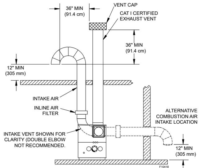
**Figure 40. Ducted Air - Vertical**
