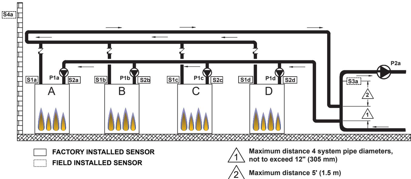
Figure 18. MODE 1 - Boiler Cascade with Primary/Secondary Piping
