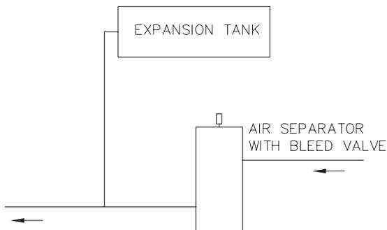
**Figure 14.** Air-Separation/Expansion Tank
