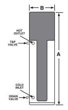
8" TOP CLEARANCE FOR AIR CIRCULATION 3/4" WATER CONNECTIONS 240 VOLT – 1 PH
