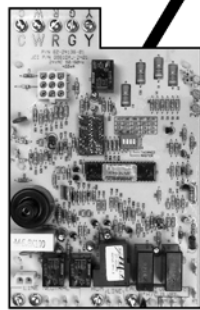
INTEGRATED FURNACE CONTROL
