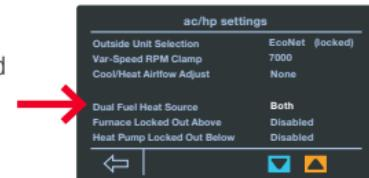
Furnace Locked Out Above: Disabled (default), 0-55 F – Outside temperature above which the furnace will not run.
