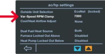
**EcoNet (locked)** – if a communicating EcoNet outdoor unit is discovered, the menu will automatically display “EcoNet” and the selection cannot be changed (locked). If no outdoor unit is present, select “none”.
